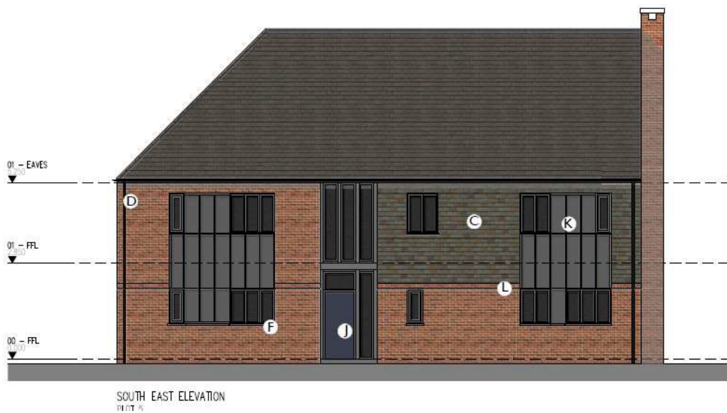
Figure 8: 'Barn-like form': Hipped roof to one side with chimney. Mostly brick with hanging tiles and fibre cement panels with plain clay tiles to roof. Powder coated composite aluminium / timber windows
